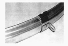
Bolt the bridge bracket to the brake bridge and slide the fender forward to the desired location. Now bolt the front of the fender to the chainstay bridge. Remember the leather washer. Pinch each side of the sliding bridge bracket with pliers to lock the fender in place and so it doesn't rattle
